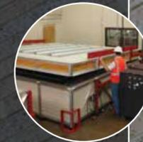
The technology in our accredited **Guarded Hot Box** is unique in the industry and includes more than 300 sensors that accurately measure and maximize the thermal performance of all our roof and wall assemblies.
